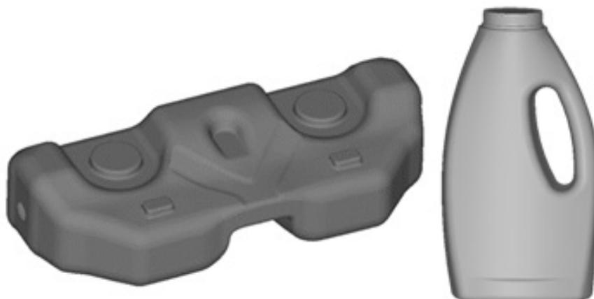
Figure 5.1: Blow moulded components
