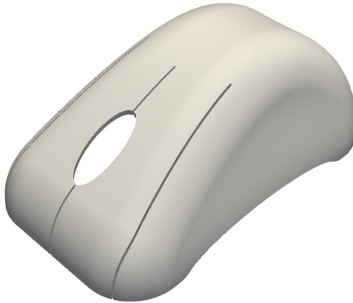
Figure 12.9: This geometry represents the outer shell of a computer mouse. For the test case, this part will be analyzed during a filling analysis using Autodesk Moldflow. The molten plastic is injected at a single injection location at the back of the mouse
