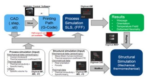
Figure 5.13: Simulation process workflow - Additive Manufacturing
