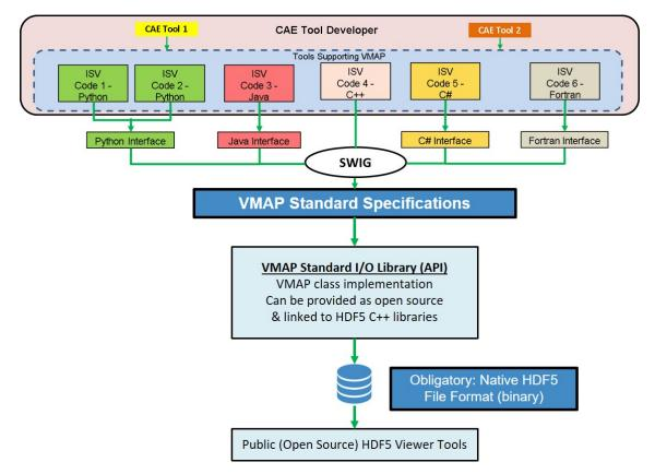
Figure 4.2: Extended VMAP Software Architecture
