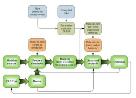
Figure 5.11: Simulation process workflow - Injection Moulding - Creep
