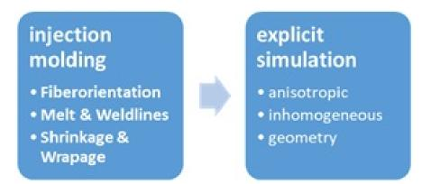
Figure 5.6: Simulation process workflow - Injection Moulding - Impact
