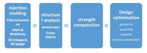
Figure 5.10: Simulation process workflow - Injection Moulding - Fatigue
