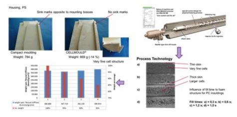
Figure 5.7: Injection Moulded Parts - Foaming
