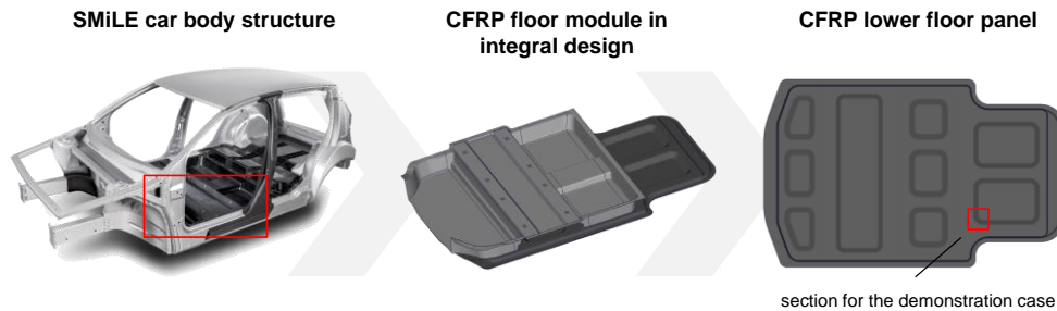
Figure 1: CFRP lower floor panel from SMiLE car body structure used for demonstrating structure.
